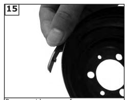
Remove side covers from canopy exposing 4 holes. 2 closed holes and 2 open "L" shape holes.
